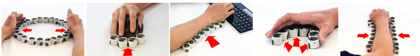
Figure 1: SwarmHaptics uses a swarm of robots to display various haptics patterns to different body parts that are on a surface or through external objects such as a mouse. It can be used to convey notifications, social touch, directional cues, etc.
