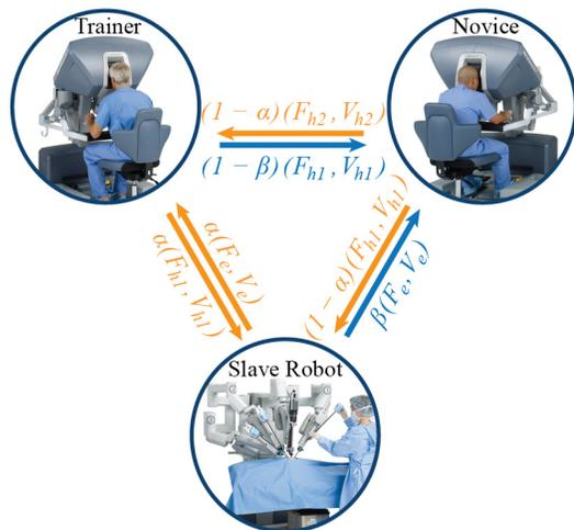
Fig. 1. Schematic shared-control architecture designed for trilateral teleoperated training robots. The inputs ( $F$ 's and  $V$ 's) to the robots are scaled using a dominance factor ( $\alpha \in [0,1]$ ) and an observation factor ( $\beta \in [0,1]$ ). Images ©2015 Intuitive Surgical, Inc.
