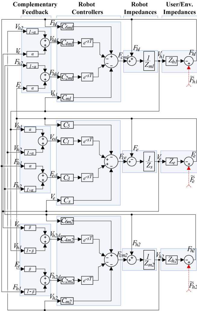
Fig. 4. Trilateral shared-control architecture. The input signal to the trainer and slave robot are gauged using the dominance factor  $\alpha$ , and the input to the novice robot is gauged using the observation factor  $\beta$ .
