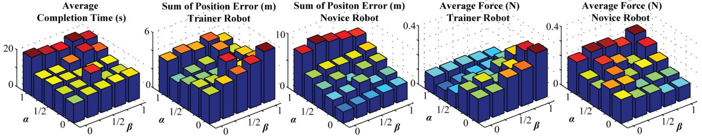
Fig. 9. Average time of completion, sum of position error (absolute value of the difference between the robots position and the trajectory) and average force magnitude for the trainer, and novice robots across different  $\alpha$  and  $\beta$  values.
