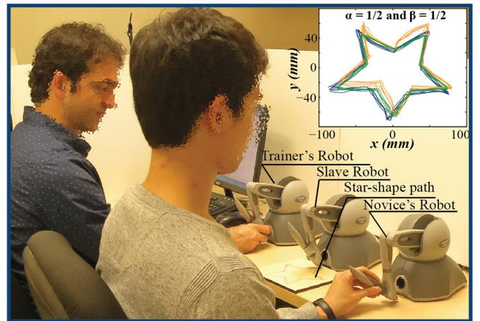
Fig. 6. A dyad of human users performed a trajectory following task. The first user was given more control and moved the stylus of his haptic device by the dominant hand (allowed to be supported on the table). The second user was the novice and moved the stylus of the haptic device using the non-dominant hand (not allowed to be supported on the table). The gimbals of the trainer and slave robots were similarly fixed using tape.
