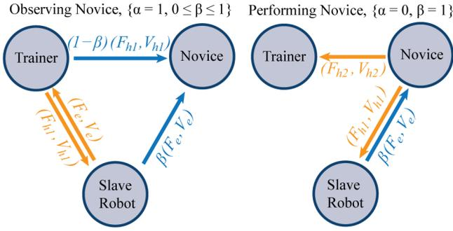
Fig. 2. Two special cases of the shared-control architecture. Left: Using  $\alpha = 1$ , the trainer is the primary performer and the novice is primarily observing the movements of the trainer ( $\beta = 0$ ) or slave ( $\beta = 1$ ). Right: Using  $\alpha = 0$ , the novice is the primary performer and  $\beta = 1$  given that  $(\alpha, \beta)$  values are chosen from  $\Omega$ . In this case, the controller gives the full control over the trainer master robot and slave robot to the novice.
